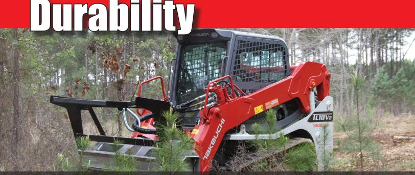
The purpose built frame features multiple cross members for greater strength and rigidity. The heavy duty step cross member protects the bucket cylinders from damage and provides better visibility to the cutting edge of the bucket. With the added strength and durability, the track loader makes an excellent attachment platform with the heavy duty lift cylinders with oversized pins and bushing that are built for greater lifting capacity and enhanced performance.
