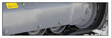
Several different track systems can be found on Takeuchi track loaders. The TL8 features steel on steel contact between the rollers and mandrels allowing abrasive material to be crushed or expelled from the track system. The TL10V2, TL12R2 and TL12V2 have a quiet ride track system that allows the rollers to ride along a rubber contact pad reducing noise and vibration levels.
