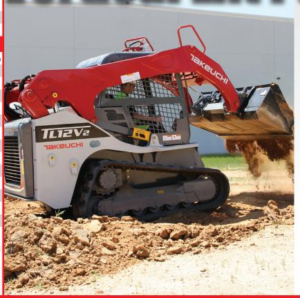
Vertical lift machines have minimal change in the loaders center of gravity because the load is kept closer to the machine throughout the lift path. They are ideal for loading trucks and hoppers with high sides and generally provide better reach at dump height.
