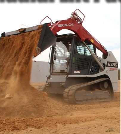
Radial lift machines feature a single arm pivot point and have higher breakout forces making them ideal for tough excavating and grading applications. They also have excellent mid-height reach which is well suited to loading and unloading flatbed trucks.
