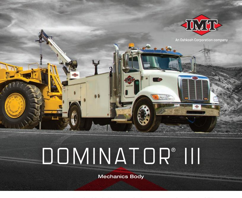
With enhanced strength and stability for higher crane loads, numerous configuration possibilities, and a body rating of 81,000 ft-lb (12.3 tm), the Dominator III mechanics truck offers exceptional performance in virtually any industry. With the Dominator III mechanics truck, you don't have to bring your equipment into the shop for service, because the shop comes to you.
