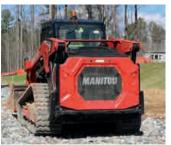
Counterweight A rear bumper counterweight improves productivity and protects the machine rear from accidental damage. Optional side counterweights can further increase operational capacity.
