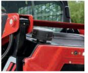
**Pre-Cleaner** Reduce engine wear and TCO in dusty environments by adding an engine pre-cleaner.
