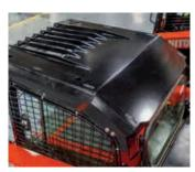
**FOPS Level 2** For the users that need level 2 FOPS an optional level 2 heavy duty bracket delivers the protection they need. Bracket also protect the front LED work lights.
