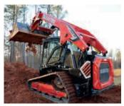
**Bucket Self-Leveling** Automatically maintain the bucket position when raising the lift arms.
